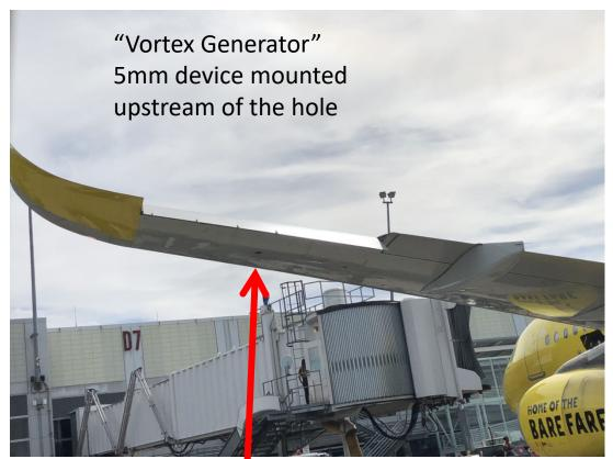
Aircraft must be taken out of service and fuel tanks & systems drained of all fuel before retrofit.
